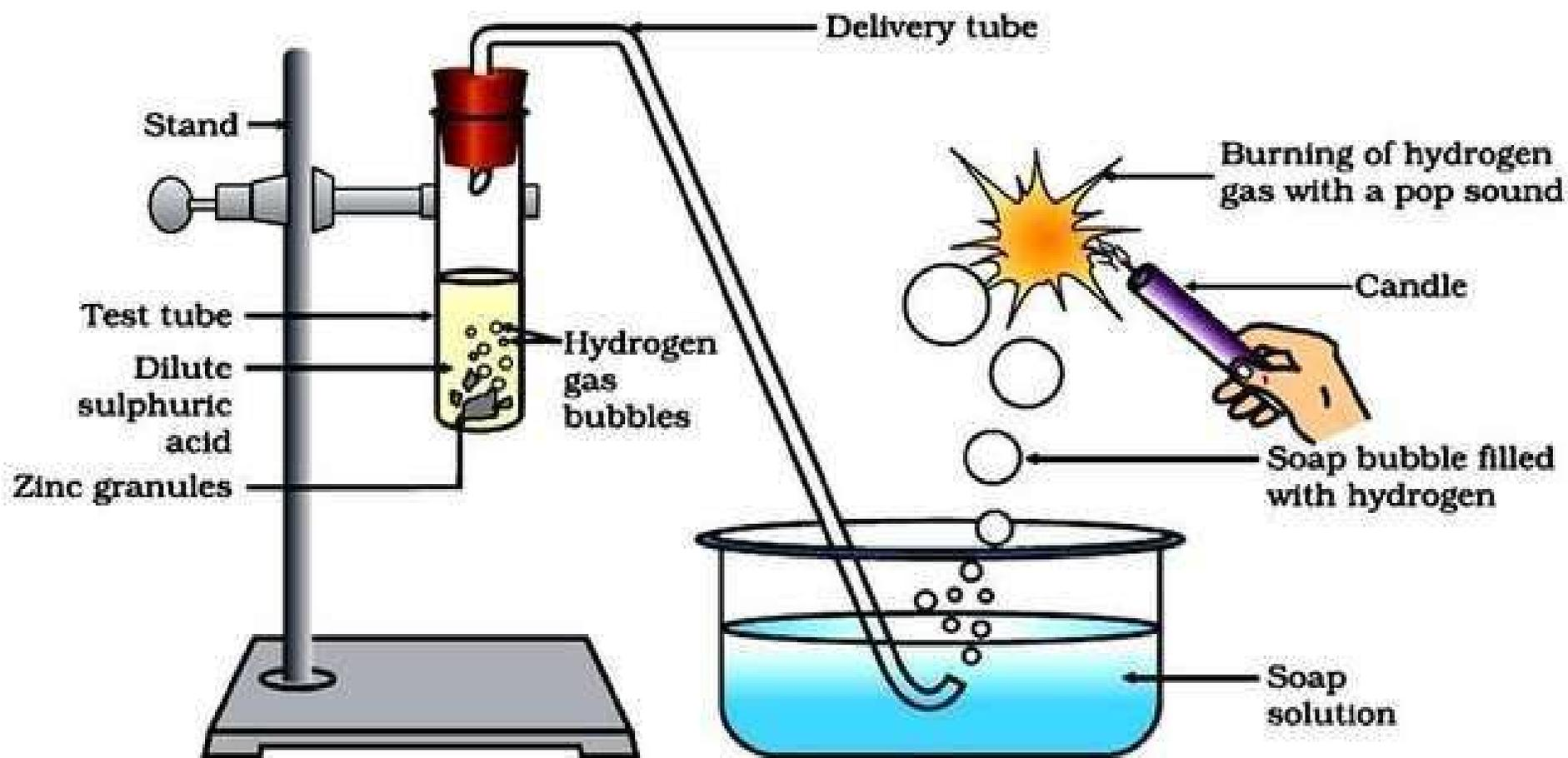
*Reaction of zinc granules with dilute sulphuric acid and testing hydrogen gas by burning*
