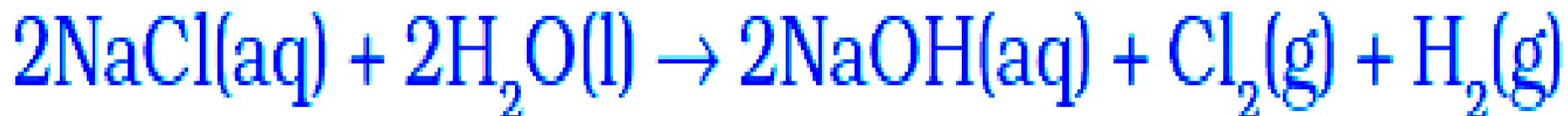
Chlorine gas is given off at the anode, and hydrogen gas at the cathode. Sodium hydroxide solution is formed near the cathode. The three products produced in this process are all useful.
