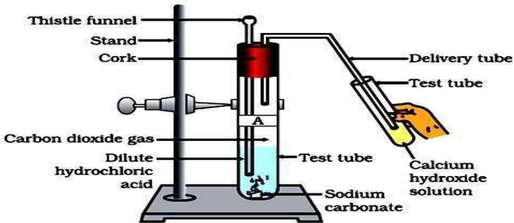
*Passing carbon dioxide gas through calcium hydroxide solution*
