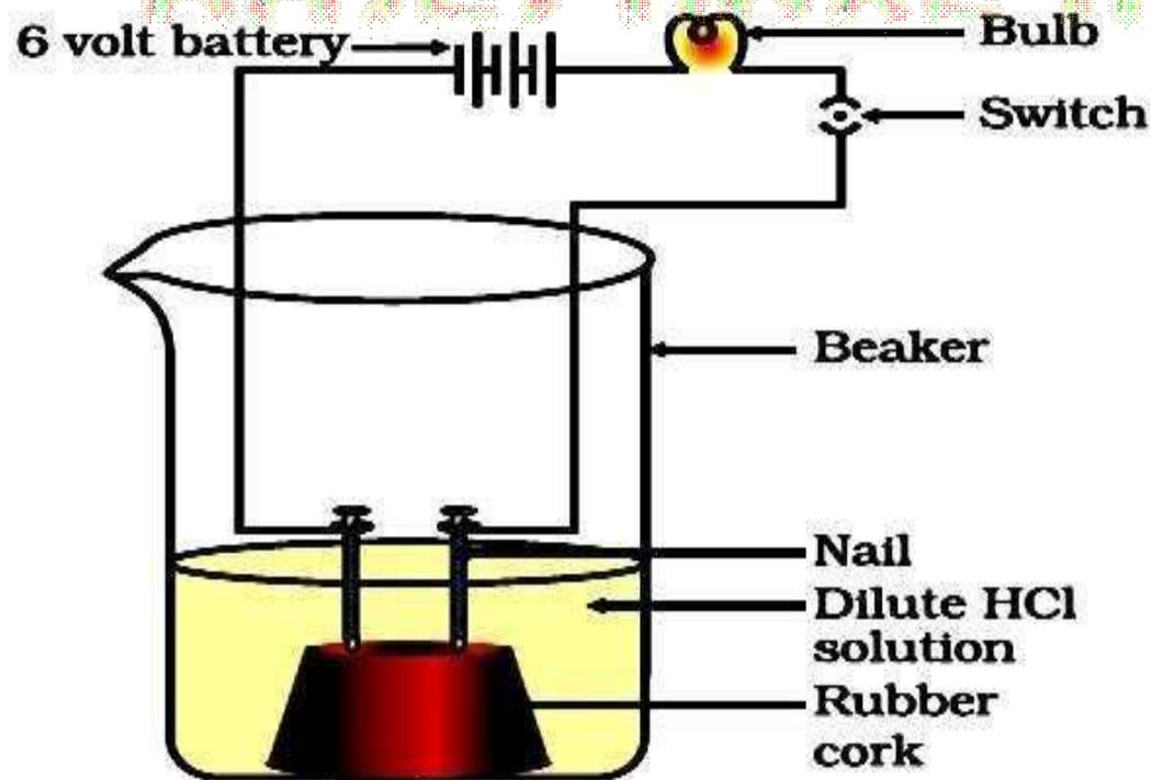
Glowing of the bulb indicates that there is a flow of electric current through the solution. The electric current is carried through the solution by ions.
